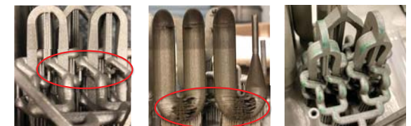
Defect due to improper support placement Defects due to improper STL processing Dye seeping through porous print material
